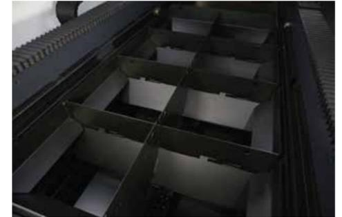
Multi-zone auto duct damper system at the table to maximize extracting fume and particles.
