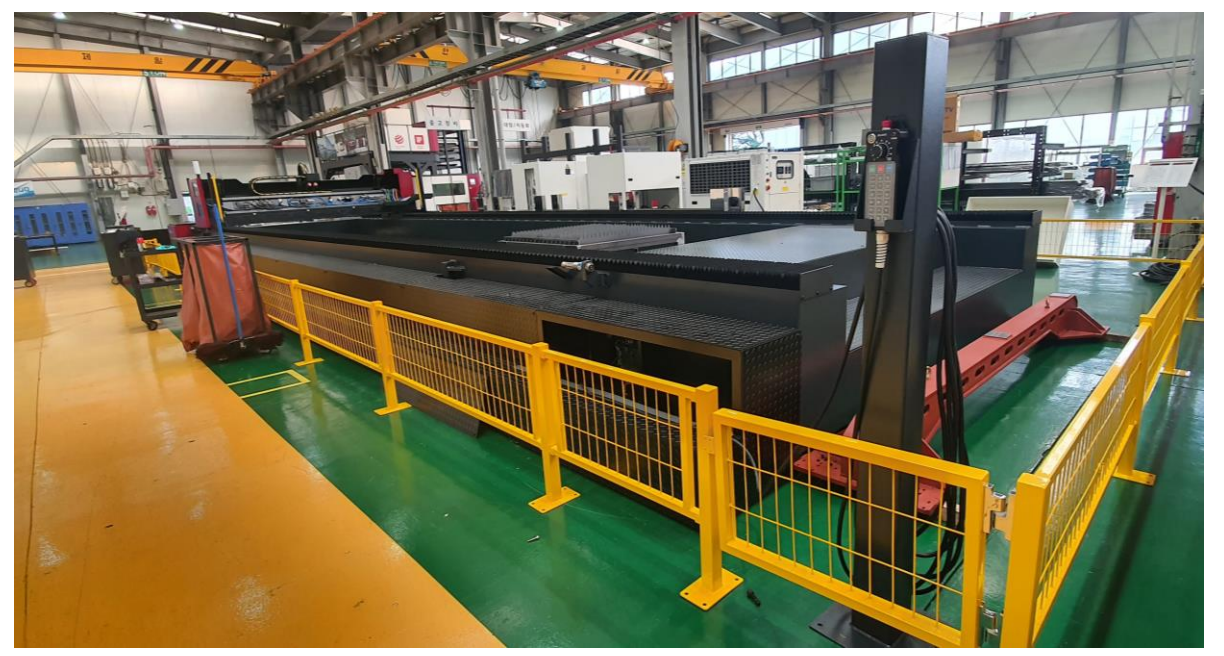
Rearview of FO 12030 Showing the dust collecting system at the side of the frame
