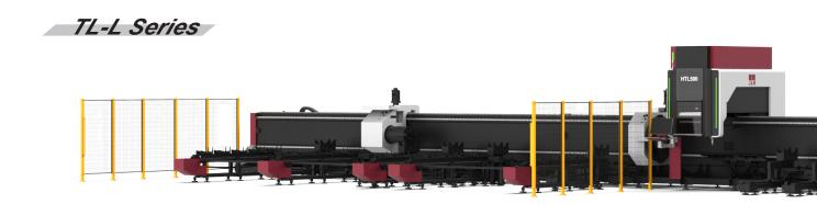
The TL-L is equipped with four chucks to facilitate heavy-duty clamping. The four chucks give the needed stability for heavy and long tubes. The maximum clamping diameter is 25.5 inches and max weight of a single tube is 2,650 pounds.
