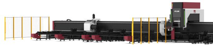
The TL-L is equipped with four chucks to facilitate heavy-duty clamping. The four chucks give the needed stability for heavy and long tubes. The maximum clamping diameter is 25.5 inches and max weight of a single tube is 2,650 pounds.
